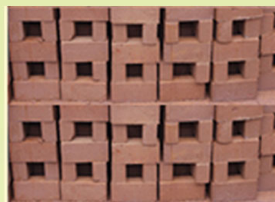
Stabilised Soil Bricks
